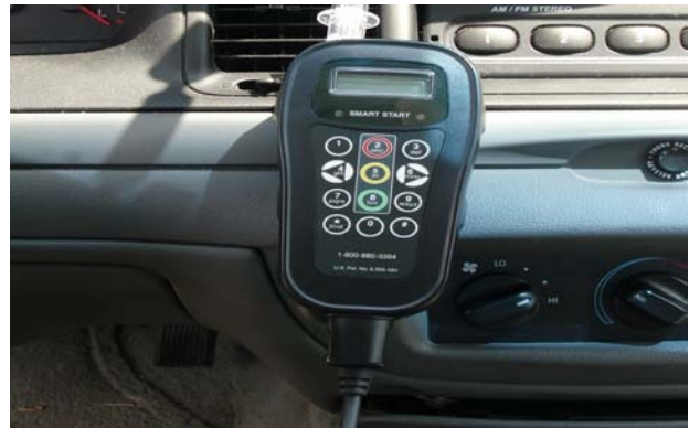
Ignition Interlock installed in auto
